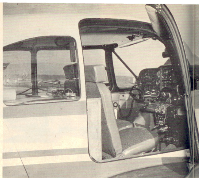
Apache One Zero Papa had plenty of fuel and instruments for the trans-Atlantic flight. Note the two 80-gallon auxiliary tanks back of the pilot's seat. A full instrument panel, plus Piper's new AutoControl automatic pilot, helped make the flight to Paris "routine"
